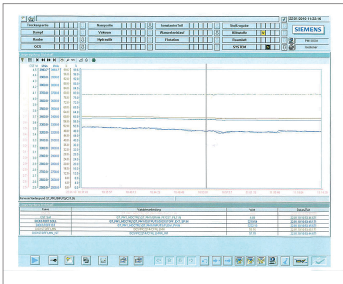
Fig. 3: Dosage metering of additives old valve (top) with strong fluctuations and new valve with precision servo motor drive (below).
